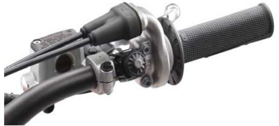
Following market investigations by KTM it has been determined that anomalies in the manufacturing process have resulted, with certain batches, in hand brake cylinders with defective machining. This can lead to early wear of the sealing cup in the hand brake cylinder, thus leading to impaired braking performance. As the anomalies are restricted to specific batches, the hand brake cylinder must be checked and the affected batches replaced.
